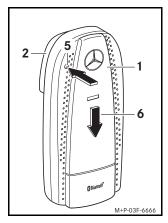
1. Press the release button (5), push the telephone module (1) down in the direction of the arrow (6) and remove it from the contact plate (2).
