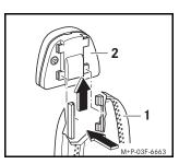
1. Press the telephone module (1) onto the contact plate (2) until it engages.
